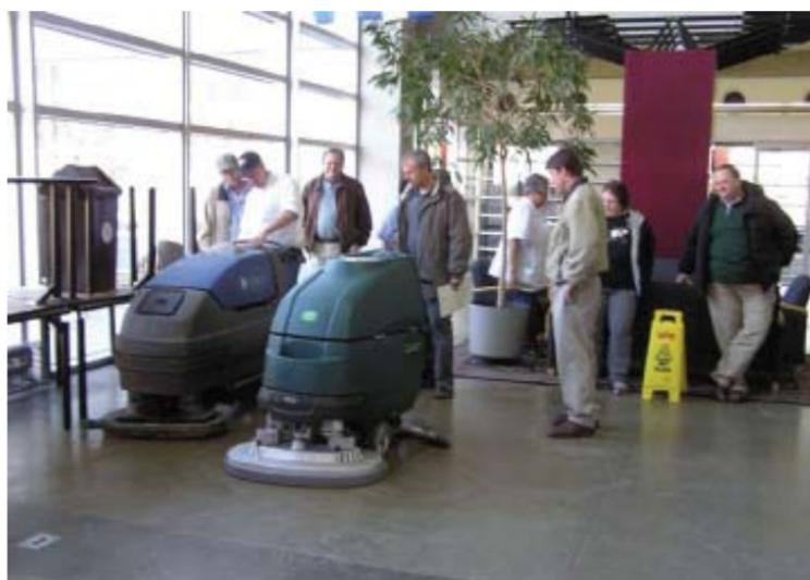
The Speed Scrub (right) challenged an older detergent-dispensing campus floor scrubber (left). The Speed Scrubber's sustainable cleaning approach, using only ionized water, won the competition and a spot in the university's fleet of more than 20 floor scrubbers. More Speed Scrub models will be added over time.
